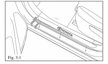
NOTE: The "TOYOTA" logo must be oriented to be read from the outside of the vehicle.
